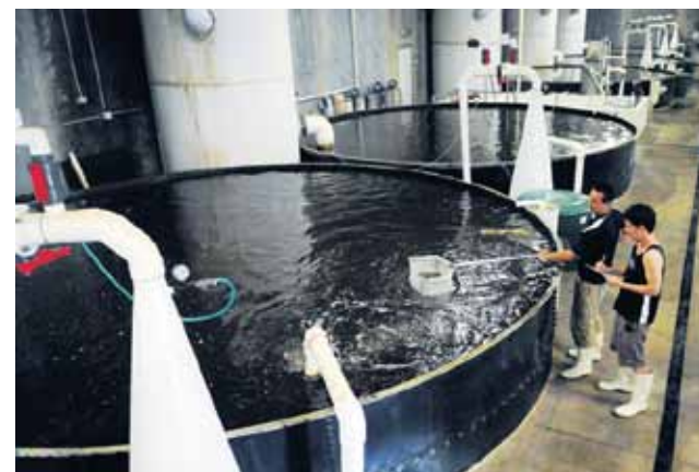
Two of Mainstream's holding tanks showing the oxygenation cones and the biofilters.
