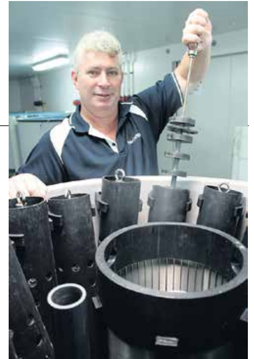
The Sep-Art machine: Artemia cysts are hatched in the main tank and the iron-infused cysts are attracted to the magnets Paul is holding. Artemia nauplii swim into the centre column and are collected and fed to the larvae.
