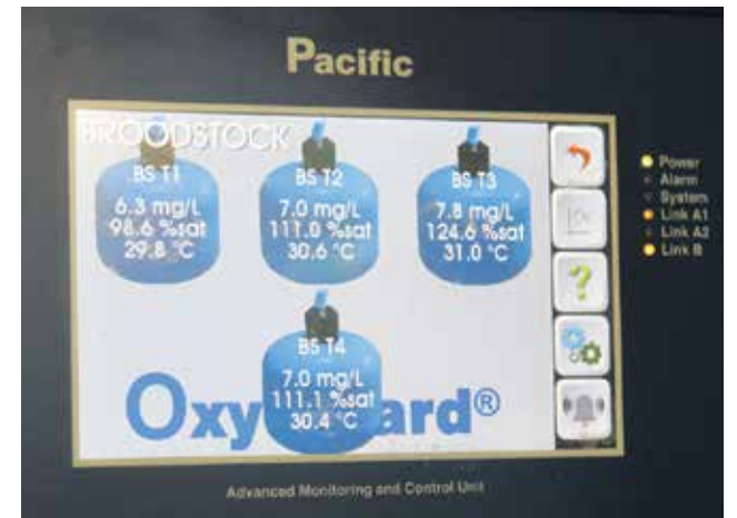
Monitor panel showing conditions in broodstock tanks.
